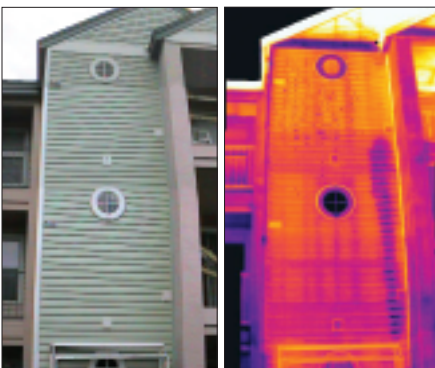
The thermogram of this vinyl-sided 3-floor apartment building clearly shows the path of a serious leak, completely hidden within the wall, from a washing machine on the third floor.
